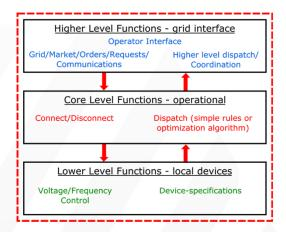
High-level example of coordination needed from higher (grid service) functions to lower level (device) capabilities.
