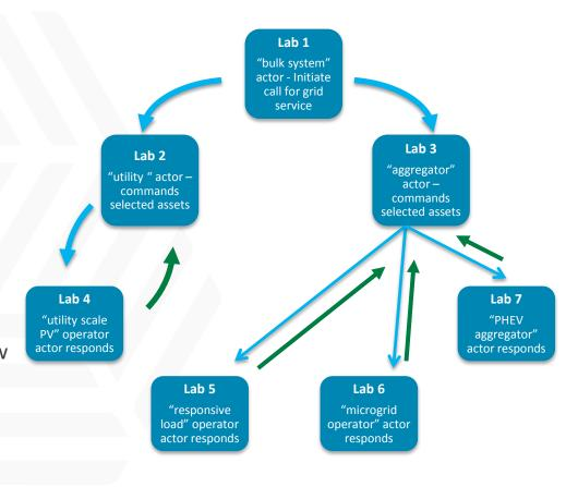
Concept of proposed demonstration of end-to-end grid service command and execution
