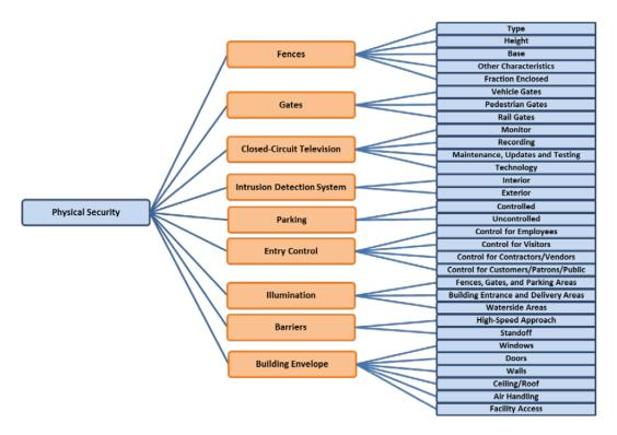
Figure 4.4. Level 2 and Level 3 Subcomponents for the Level 1 Physical Security Component (Argonne 2013)
