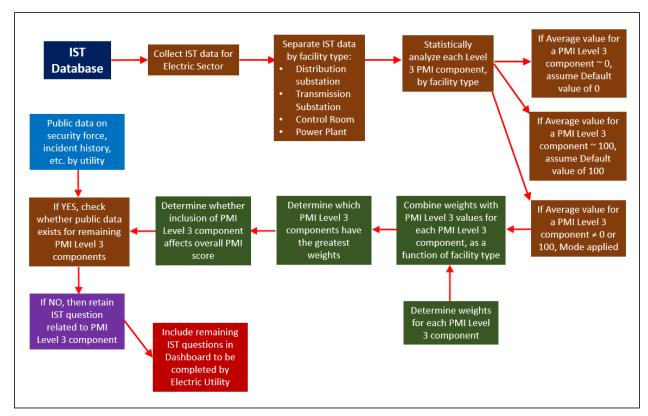
Figure 4.3. Overall Process Diagram for Revising the DHS PMI (Based on IST Questions) for the Electric Sector
