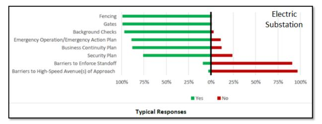
Figure 4.11. Typical Responses to IST Questions for Electric Substations
