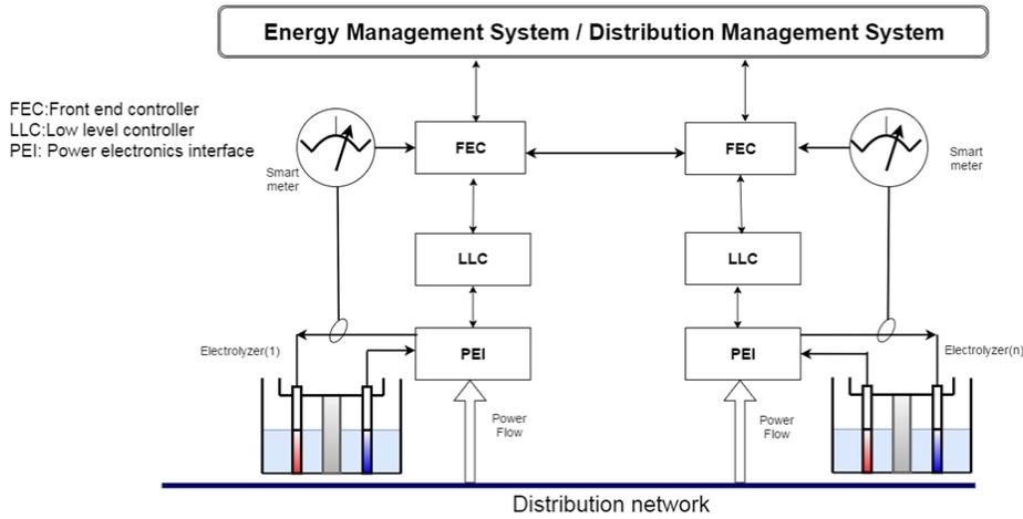
Figure F.3. Front-end controller system architecture.
