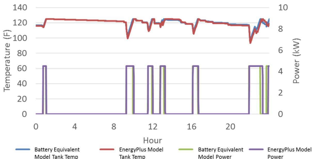
Figure A.2. Water heater tank temperatures and energy consumption in the device model and EnergyPlus.
