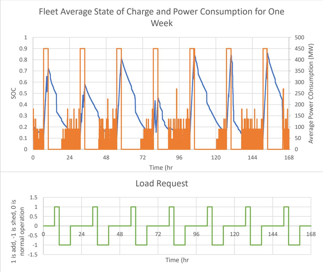
Figure A.3. Fleet average state of charge and power consumption for one week and the load request.
