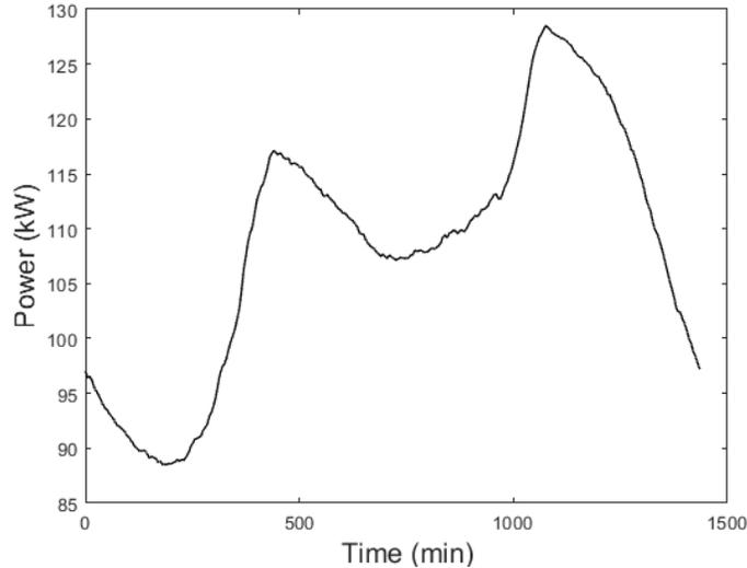
Figure F.6. Load profile used for the electrolyzer model.
