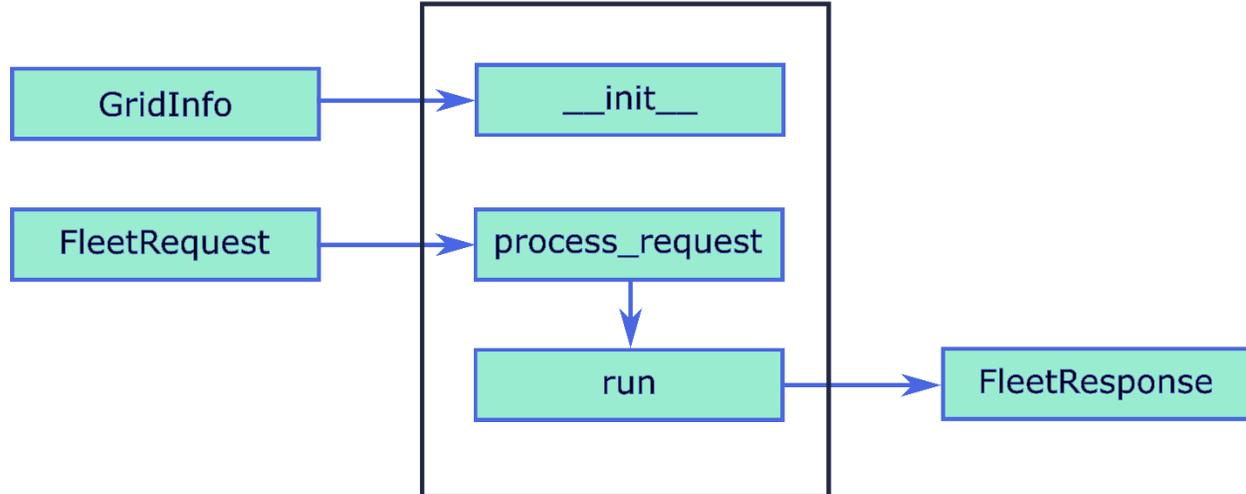
Figure F.9. ElectrolyzerFleet Class method diagram
