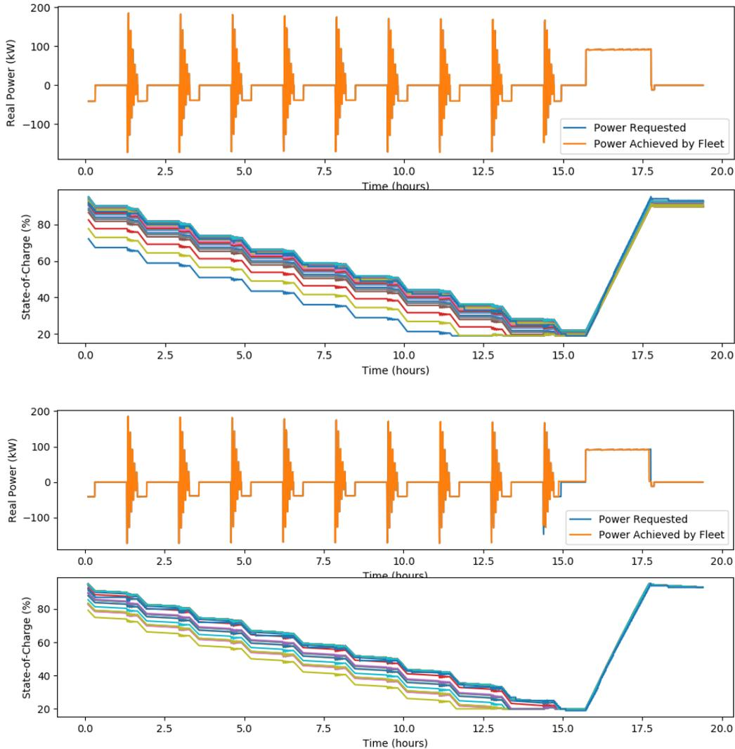
Figure D.6. Fleet Model Validation Simulation Test results of 30 battery-inverter devices using the ERM model (top) and CRM model (bottom).
