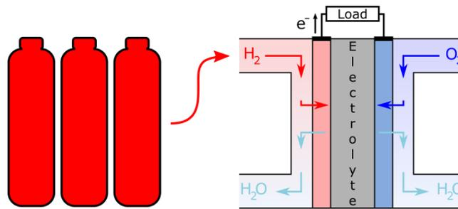
Figure E.1. Unit cell – principle of operation.
