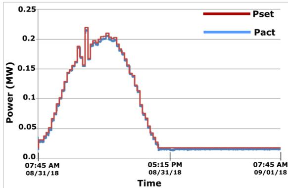
Figure F.7. Request and response with 20% renewable penetration for one electrolyzer distributed in the power system simulation.
