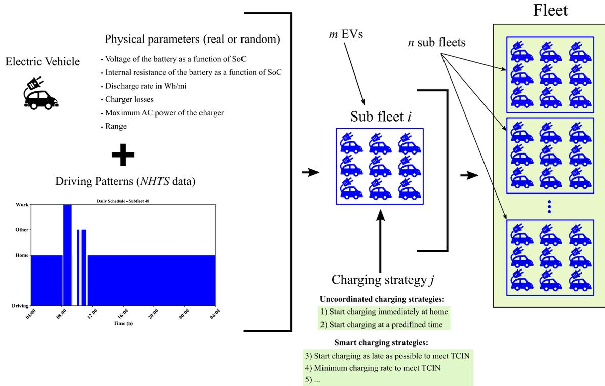
Figure B.4. Schematic of the mesoscopic model considered in this model. The physical parameters are taken from the electric vehicle model and along with the daily schedule, the sub-fleet is created, which is the minimum component of the model. Then, each sub-fleet is associated with a charging strategy to populate the fleet of EVs.
