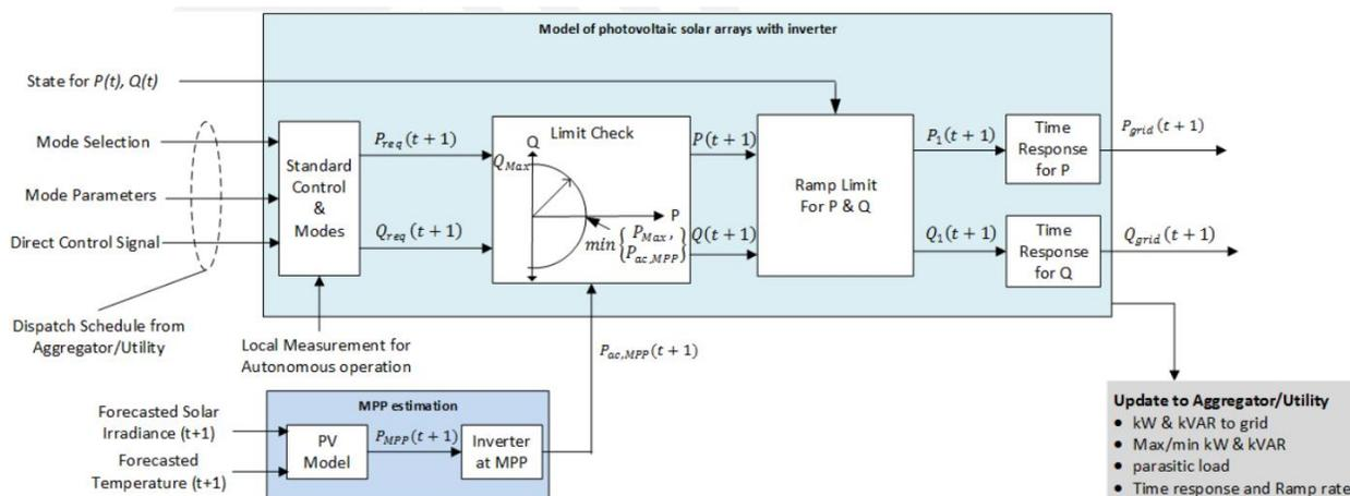
Figure C.1. Model of photovoltaic solar arrays with inverter for grid services.
