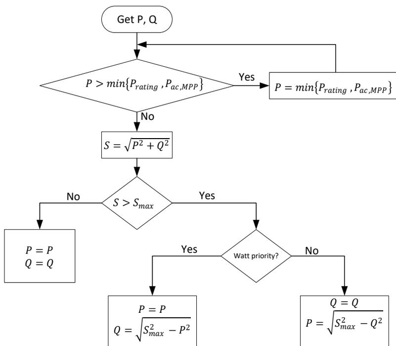
Figure C.3. Flow diagram for detection and correction of any limit violation.
