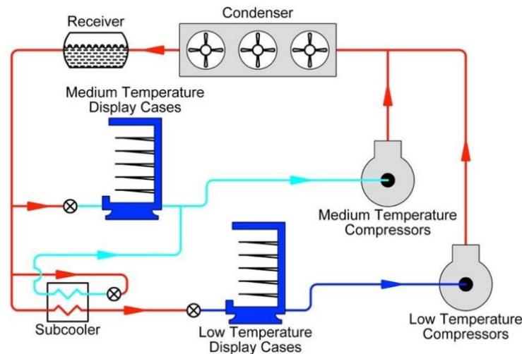
Figure H.1. A laboratory-scale supermarket refrigeration system.
