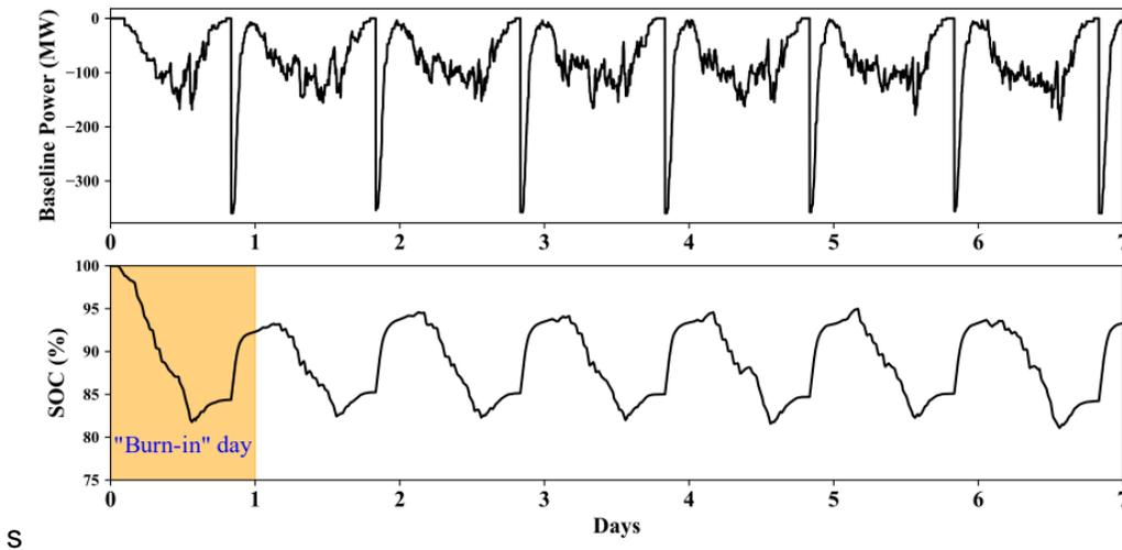
Figure B.7. Aggregated baseline power to the grid and SoC of a fleet of 200,000 BEVs as functions of time. Weights are:  $w_1 = 0.4$ ,  $w_2 = 0.3$ , and  $w_3 = 0.3$ .
