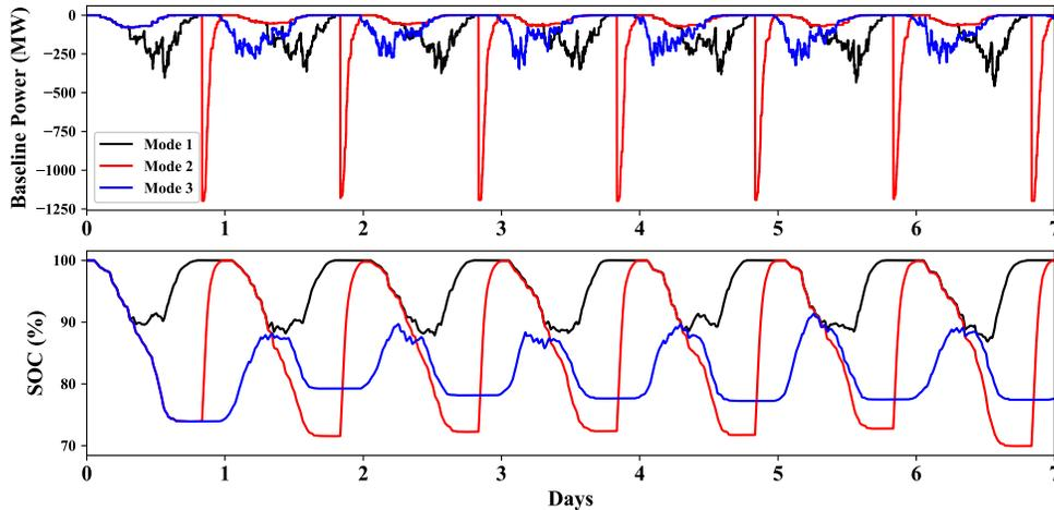
Figure B.6. Baseline power demanded to the grid and SoC of a fleet of 200,000 BEVs as functions of time.
