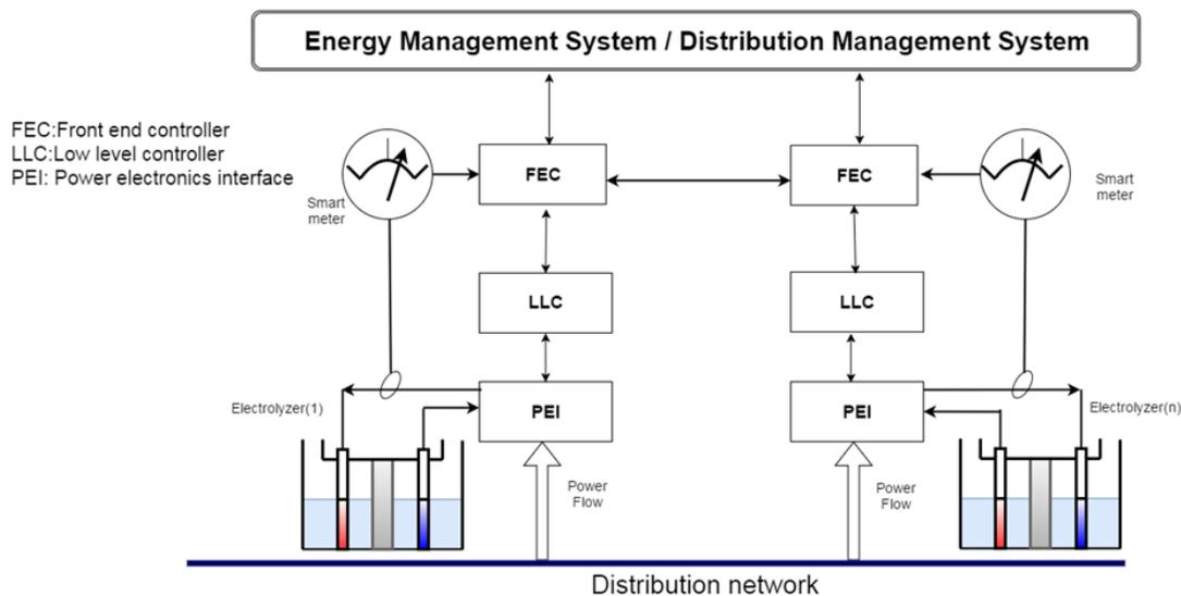
Figure E.2. Front-end controller system architecture.
