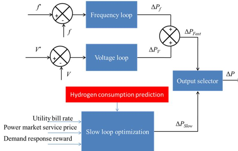
Figure E.3. Front-End Controller Control Flow Diagram.
