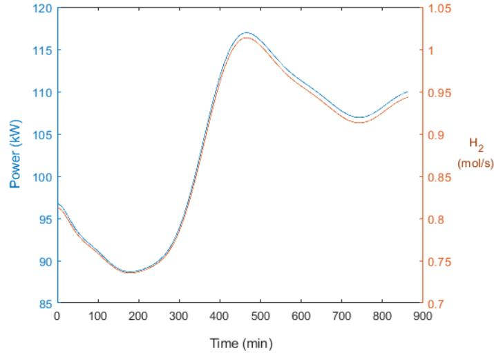
Figure E.6. Hydrogen consumption rate and power generation.
