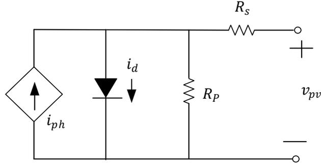
Figure C.4. Single diode model of a PV module.
