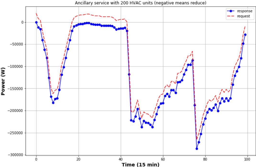
Figure G.4. Typical grid services with the HVAC fleet.
