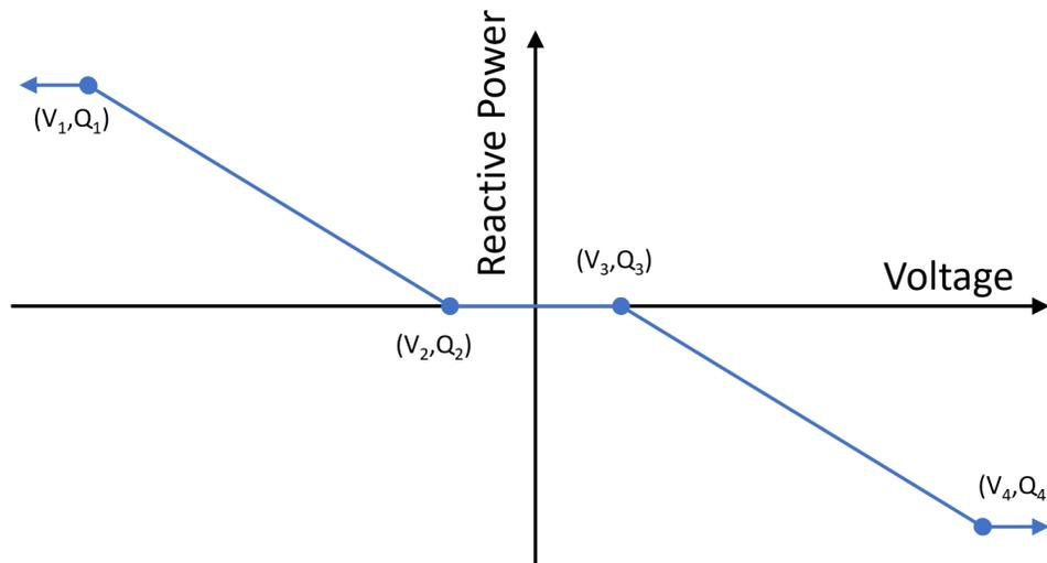
Figure D.1. Autonomous volt/var function example curve.
