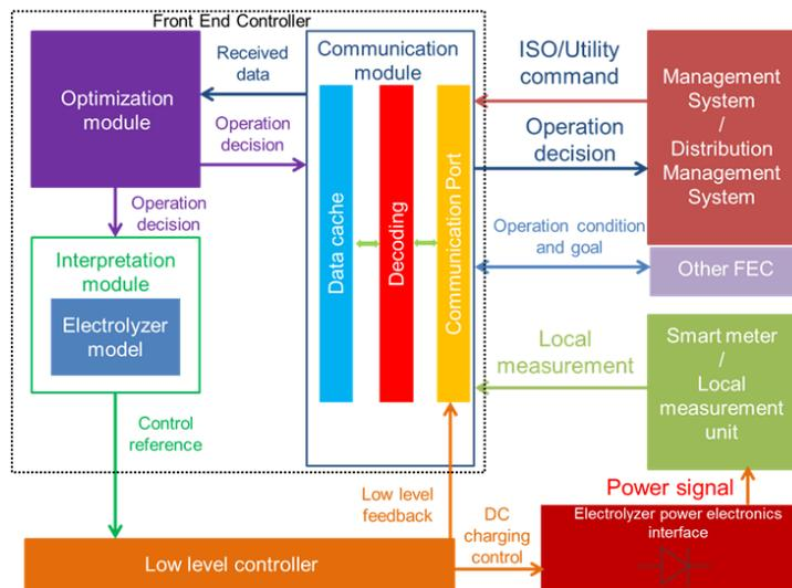
Figure F.4. Front-end controller control architecture.
