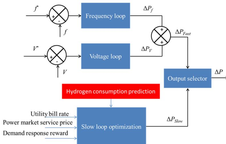
Figure F.5. Front-end controller control flow diagram.
