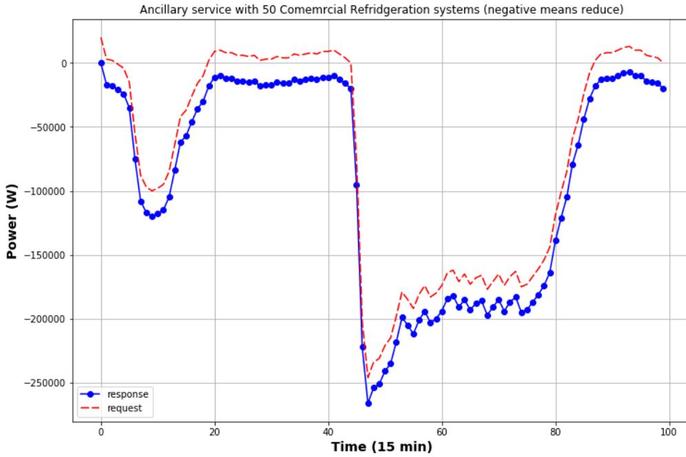
Figure H.6. Typical grid services with a commercial refrigeration fleet.
