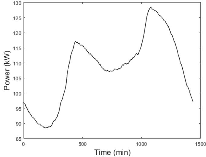
Figure E.4. Load profile used for the fuel cell model.
