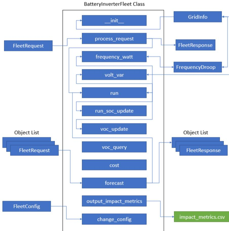
Figure D.4. `BatteryInverterFleet` class method diagram.
