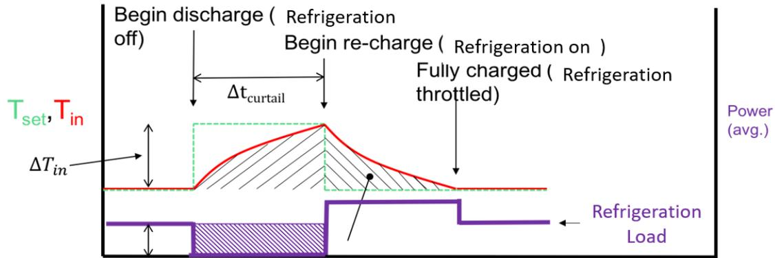
Figure H.4. Characterization of display case SoC.
