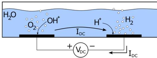
Figure F.1. Electrochemical cell – principle of operation.
