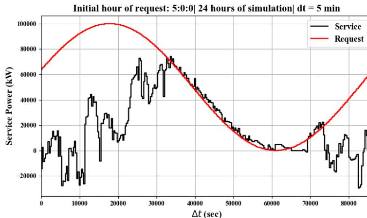
Figure B.9. Response to a 24-hour dummy grid service request. The red line represents the request as a function of time and the black line represents the service power provided by the fleet.
