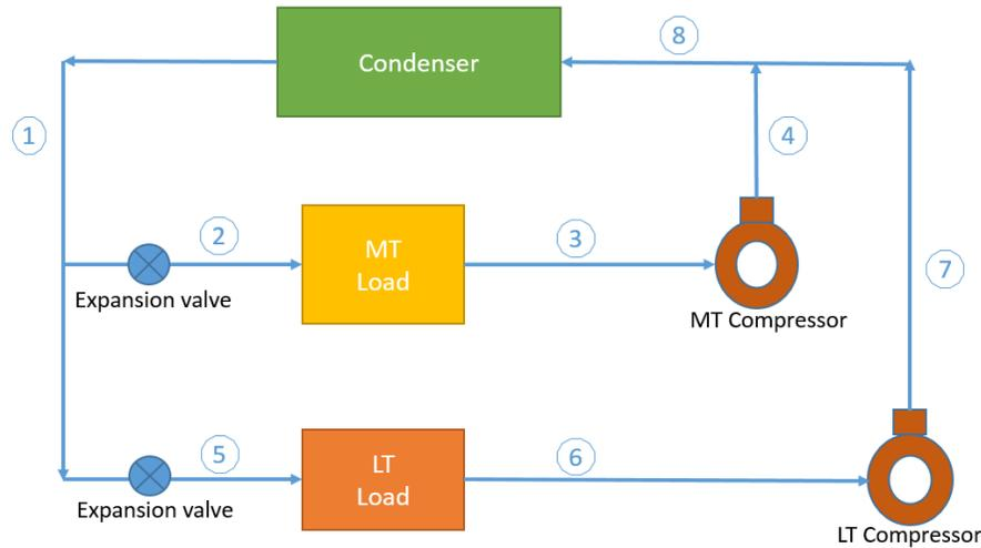
Figure H.2. Components of a supermarket refrigeration system.
