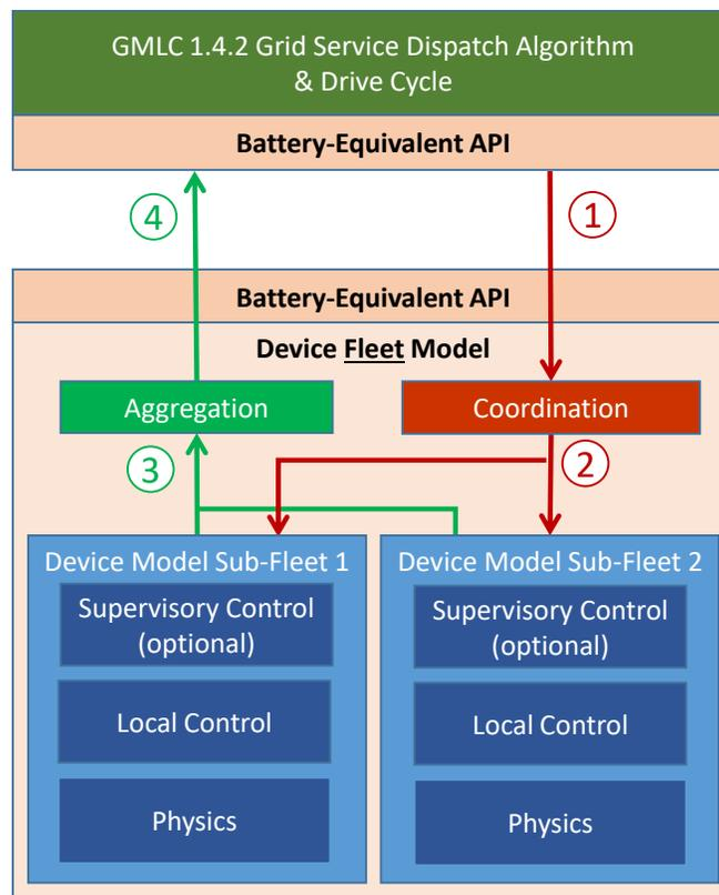
Figure 3.1. Architecture of device and device fleet models.
