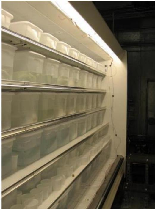
Figure H.3. Medium temperature display case in test chamber.
