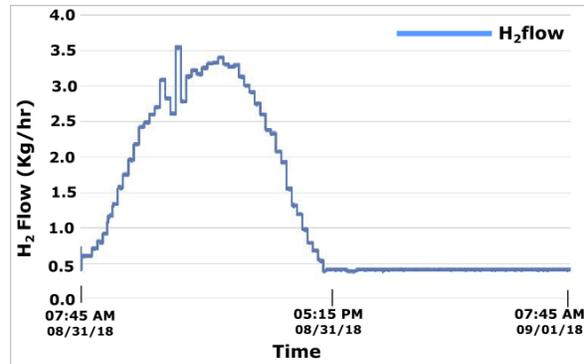
Figure F.8. Hydrogen flow for one electrolyzer.
