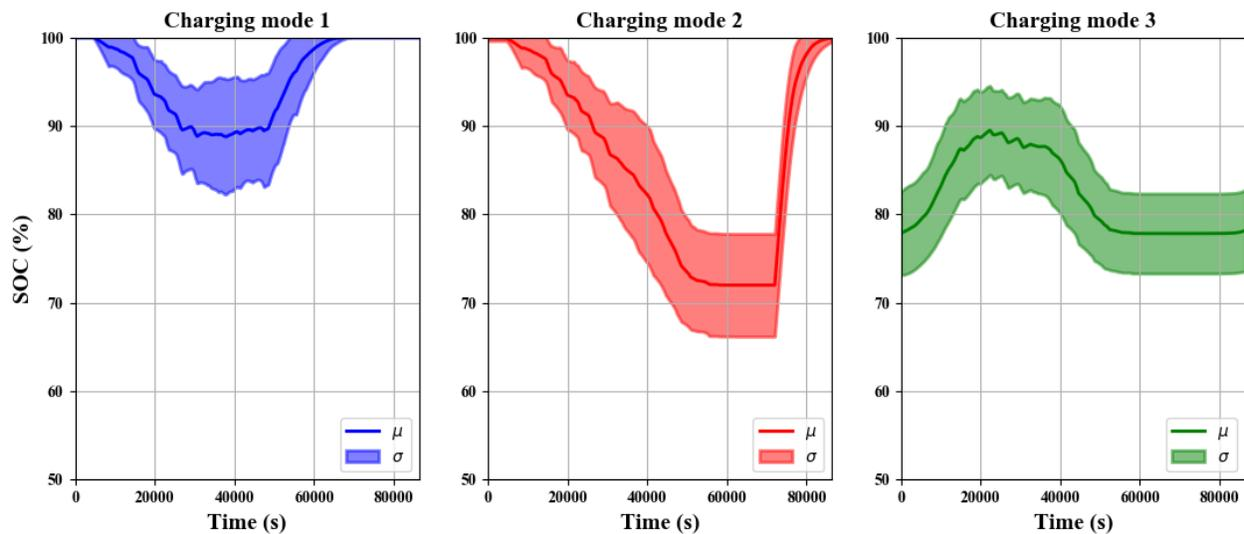
Figure B.8. The state of charge of the fleet and standard deviation as a function of time for the three charging modes considered in the model. Note that  $t = 0$  sec corresponds to 4 a.m.
