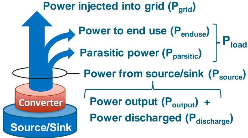
Figure 3.2. Energy balance and power flows in a generic device fleet.
