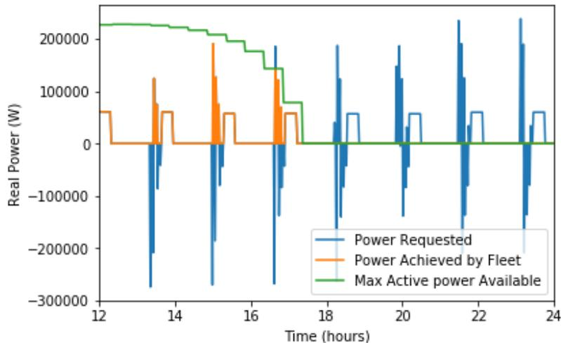
Figure C.5. Simulation result of 1,000 units of PV systems grouped together to form a PV fleet.
