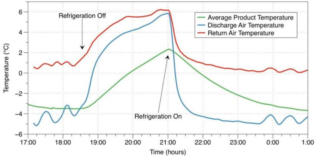
Figure H.5. Product and air temperatures in a medium temperature refrigerated display case.
