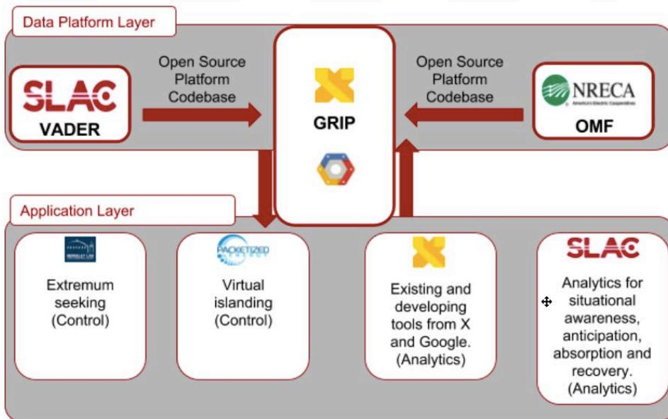
The Data Platform Layer integrates grid-related databases. The Application Layer contains the controls and analytics for event anticipation, absorption, and recovery. The two layers work together to help operators anticipate, respond to, and recover from extreme events.
