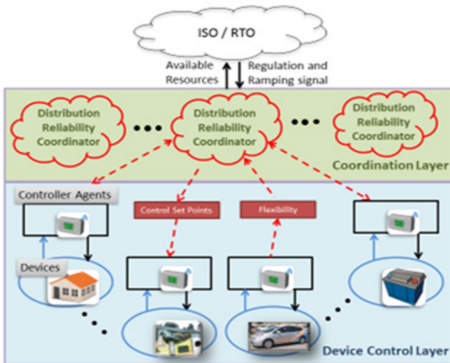
Candidate hierarchical distributed control architecture based on future distribution reliability coordinator model
